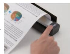
5 The page is scanned. Press the Scan button to end the scanning process and create the PDF image file.
